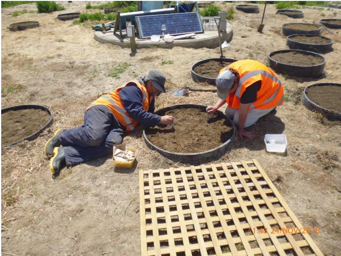
Figure 4. Lucerne seeds being hand planted to lysimeters.
